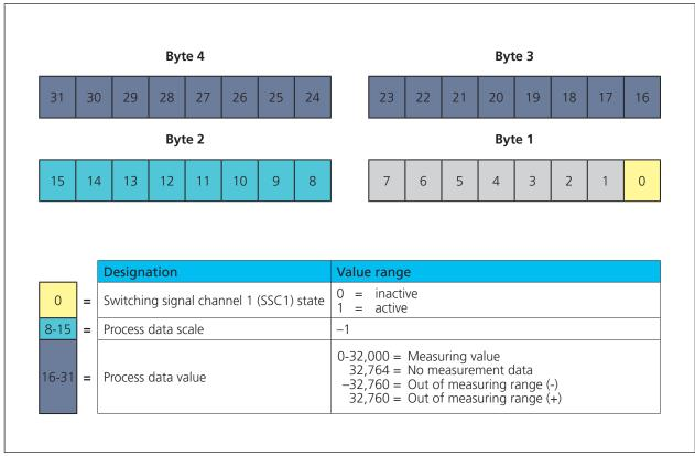
Fig. 4: Process data structure
