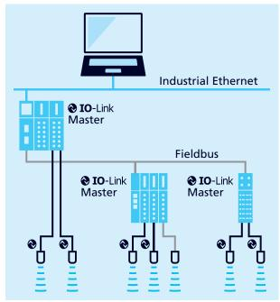
Fig. 1: Structure of an IO-Link system
