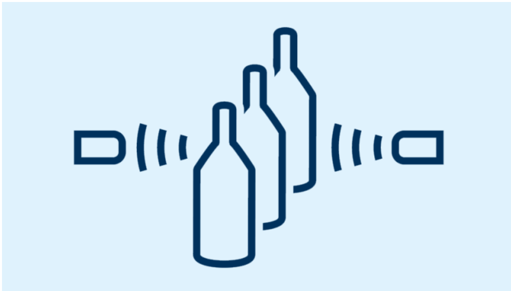
The functional principle ultrasonic through-beam barrier
