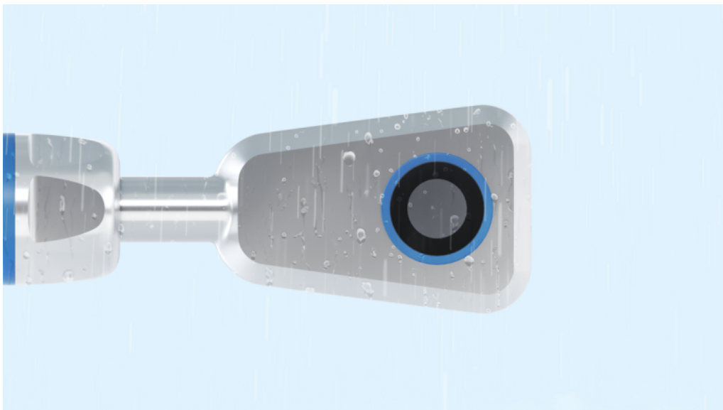
Stainless-steel sensor in wash-down design, all horizontal surfaces are at least inclined by 3^\circ
