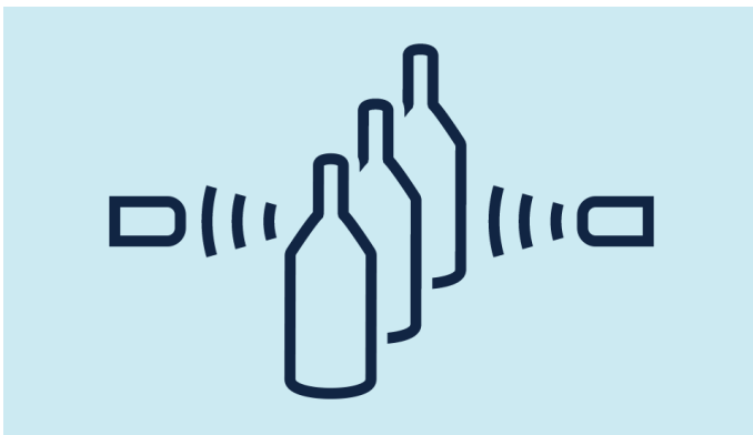
The functional principle ultrasonic through-beam barrier
