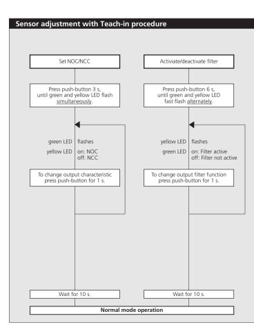
With the Teach-in procedure the response time and an off-delay can be set to 5 ms.
