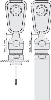
Fig. 5: pms sensor D12 adapter shaft with sensor screw connection BF-pms/A1 mounted to machine part or to stainless steel tube D26.8 with internal thread M20x1.5
