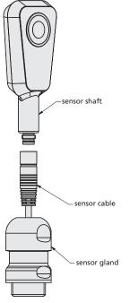
Fig. 4: Mounting of pms sensor with sensor screw connection BF-pms/A1
