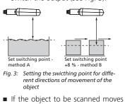
into the detection area from the side, the »Set switching point +8 % - method B« Teach-in procedure should be used. In this way the switching distance is set 8 % further than the actual measured distance to the object. This ensures a reliable switching behavior even if the height of the objects varies slightly (see Fig. 3).
