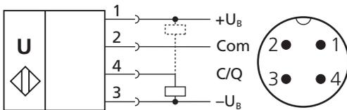
Fig. 3: Connection diagram of the nano sensor
