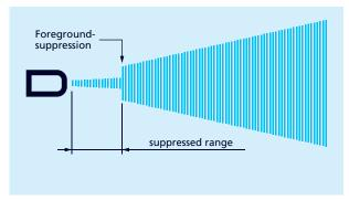
Fig. 13: Measurement configuration – foreground suppression
