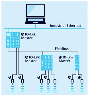
Fig. 1: Structure of an IO-Link system
