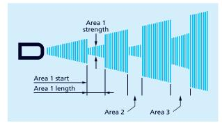
Fig. 15: Setting options for the interference echo suppression
