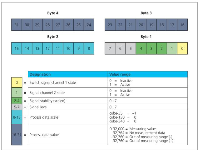
Fig. 4: Process data structure
