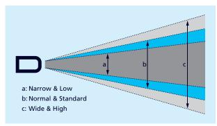
Fig. 12: Setting options for the detection area
