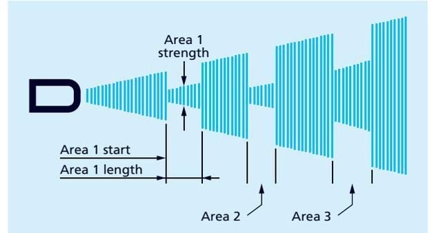
Fig. 15: Setting options for the interference echo suppression
