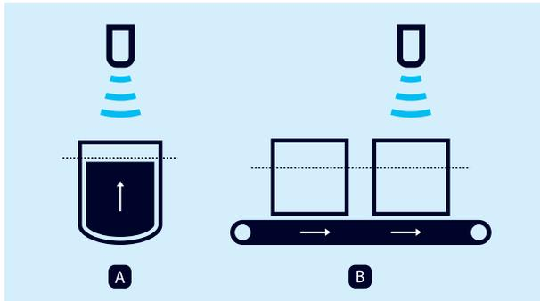
Fig. 5: Switching point mode of the sensor, Method A and B
