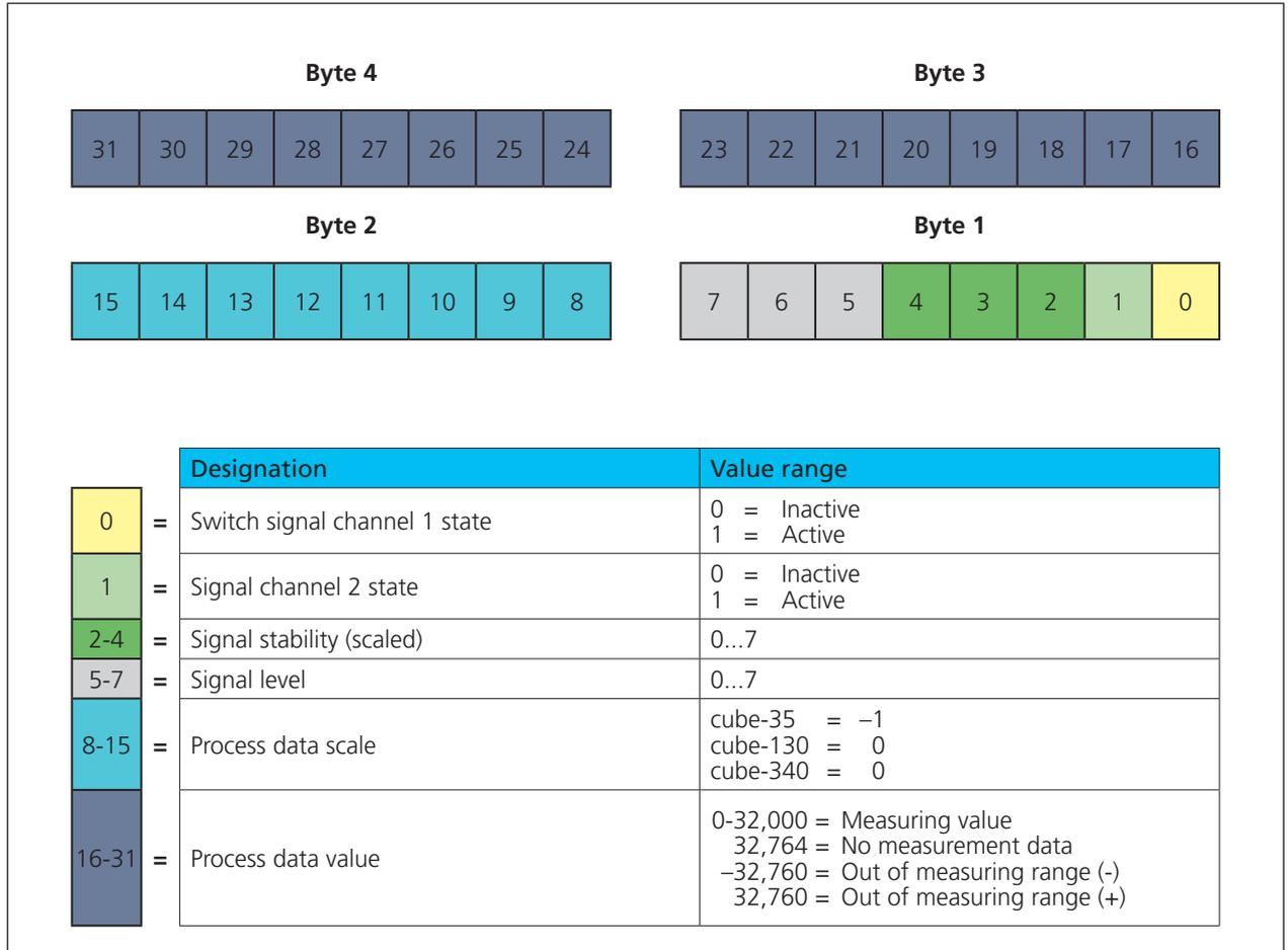
Fig. 4: Process data structure
