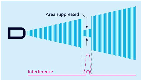
Fig. 14: The principle of interference echo suppression
