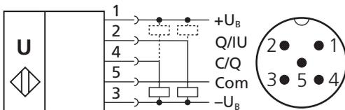
Fig. 3: Connection diagram of the cube sensor
