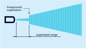
Fig. 12: Measurement configuration – foreground suppression
