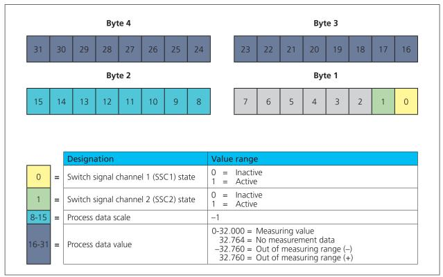
Fig. 4: Process data structure
