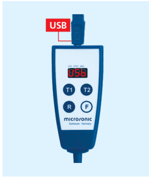
USB interface for PC connection
