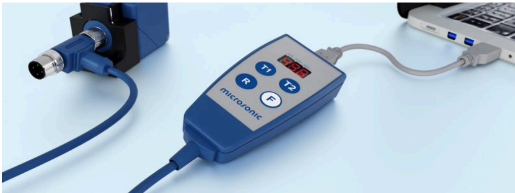
cube sensor connected to the PC via LCA-2 for programming
