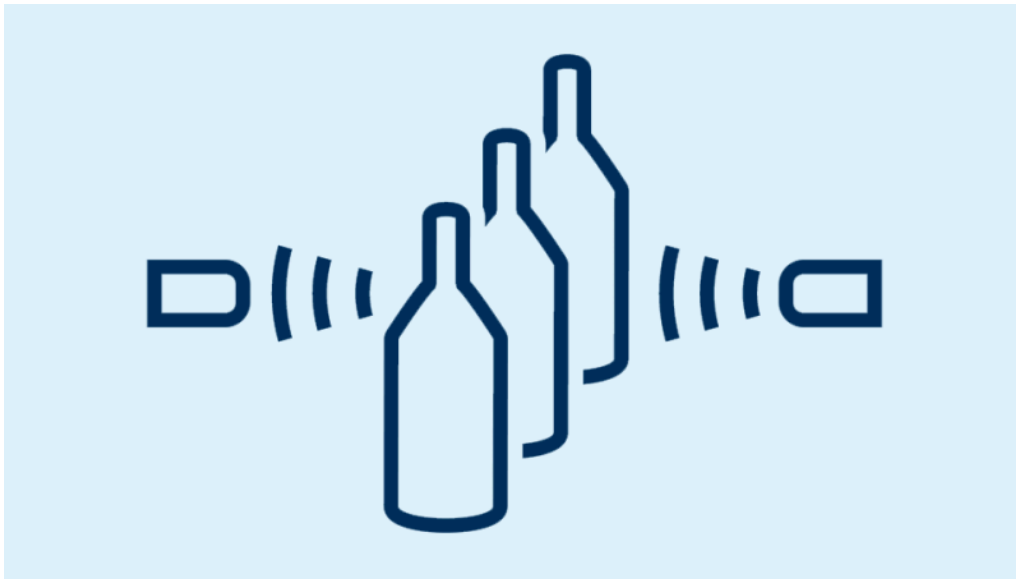
The functional principle ultrasonic through-beam barrier
