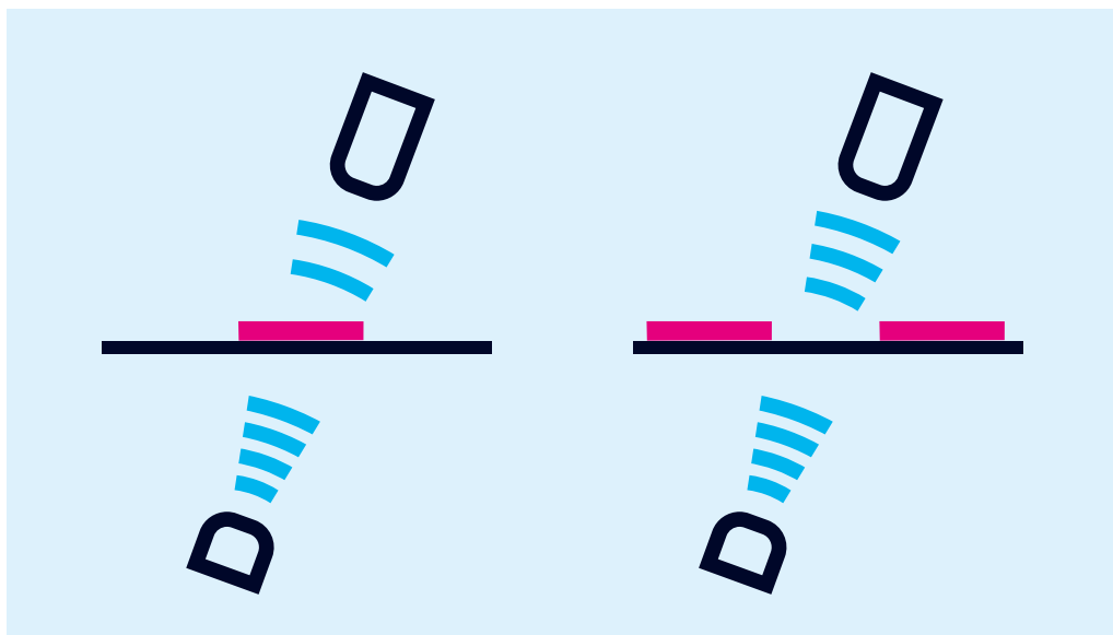
Backing material with label provides an attenuated signal level
