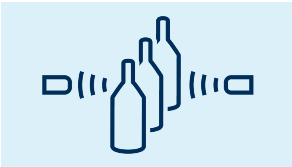
The functional principle ultrasonic through-beam barrier
