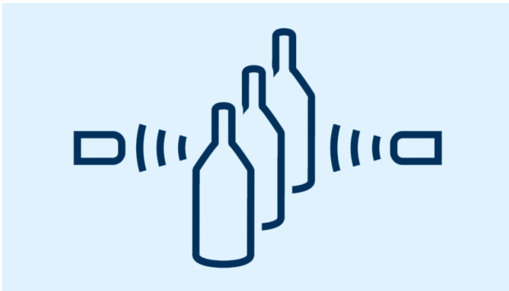
The functional principle ultrasonic through-beam barrier
